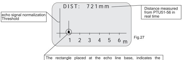
The rectangle placed at the echo line base, indicates the measurement range within which the echo signal in reception is considered always valid for the distance measurement. This interval value is variable depending on the measurement
